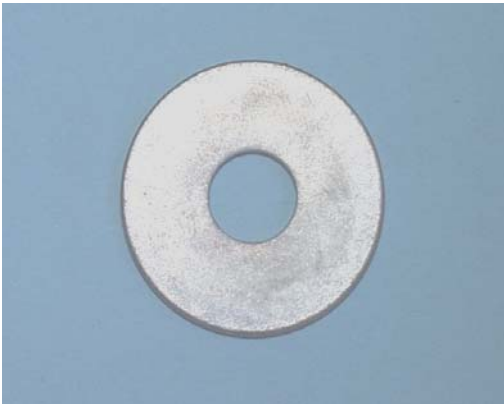
Figure 3. A sample with an electrolytic zinc plating, as received from the manufacturer. It appears to be a good magnet.
