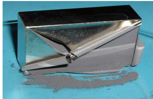
Figure 2. A sample with Ni-plating after 20 hours of a HAST at 130°C, 260 kPa and 95% humidity. Note that the plating has peeled away from the magnet.
