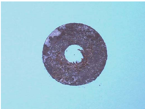
Figure 4. The same sample after 24 hours of a HAST at 130°C, 270 kPa and 100% humidity. The test demonstrates the plating was poorly applied.
