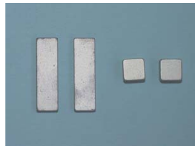
Figure 5. Samples with a spray coating after 12 days of a HAST at 130°C, 270 kPa and 100% humidity.
